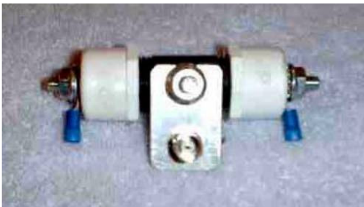
Figure 11: Completed feedpoint insulator
