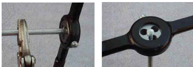
Figure 13: Cutting the threads
