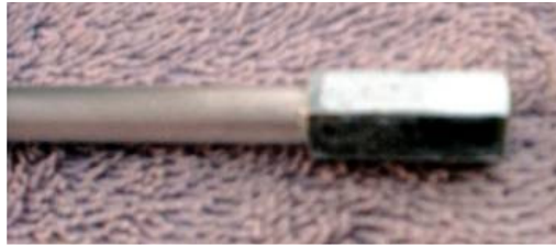
Figure 7C: Rod and coupling
